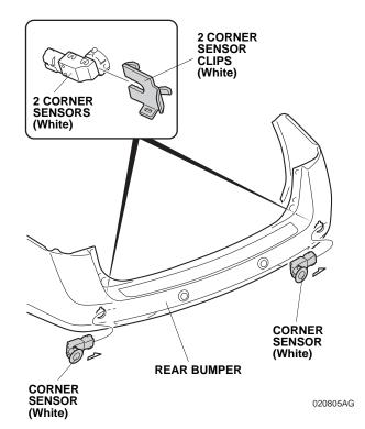
24. Secure two corner sensors (White) with two corner sensor clips (White) as shown.
