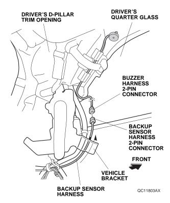
47. Plug the backup sensor harness 2-pin connector to the buzzer harness 2-pin connector.
