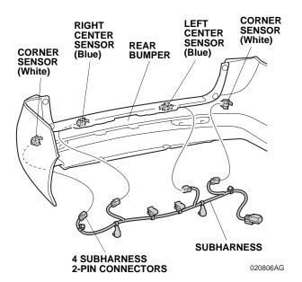
26. Secure two subharness clips to two corner sensor clips (White) as shown.
