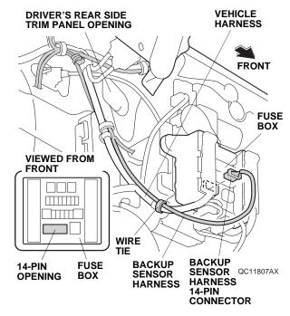
53. Secure the backup sensor harness to the vehicle harness with one wire tie. Go to step 56.
