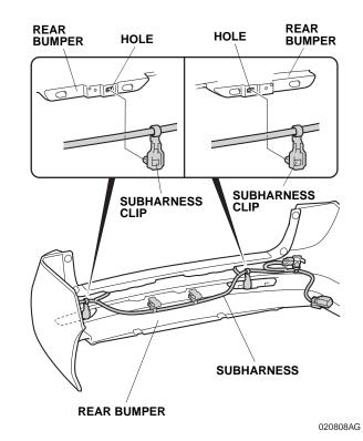
28. Secure two subharness clips to two ribs on the rear bumper as shown.
