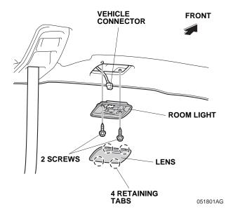
9. Remove the map light (two screws and unplug the vehicle connector).
