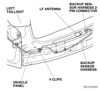
68. Plug the backup sensor harness 2-pin connector to the LF antenna.
