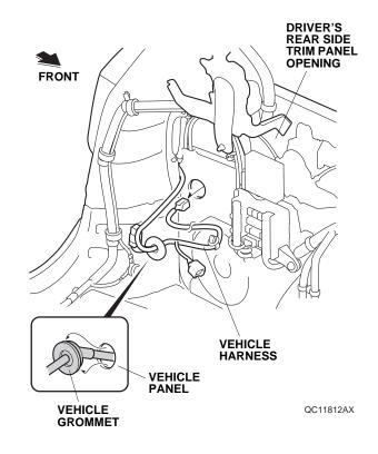
64. Route the backup sensor harness through the hole, and secure the grommet on the backup sensor harness to the vehicle panel as shown. NOTE: Do not pull on the backup sensor harness.
