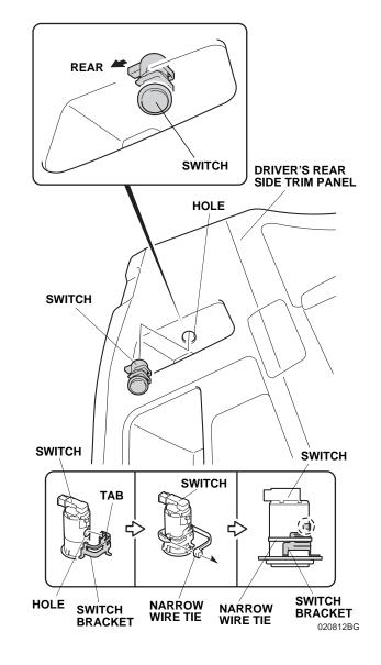
35. Align the tab on the switch bracket to the hole on the switch and secure the switch bracket to the switch with one narrow wire tie.
