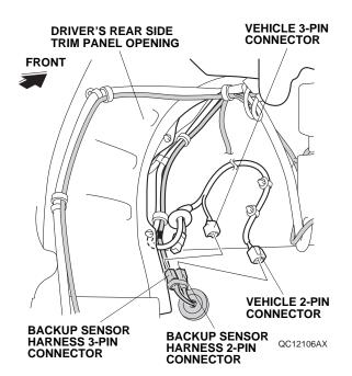
72. Plug the vehicle 2-pin connector to the backup sensor harness 2-pin connector.
