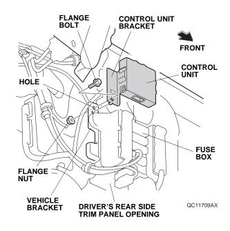
59. Route the backup sensor harness 14-pin connector, and plug it to the control unit.
