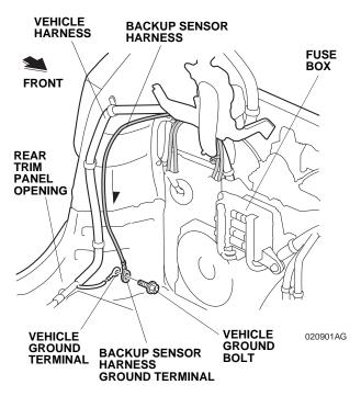
44. Remove one vehicle ground bolt and secure the backup sensor harness ground terminal to the vehicle ground terminal with the vehicle ground bolt just removed.
