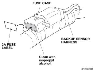
42. Secure the backup sensor harness to the vehicle harness with one wire tie as shown.
