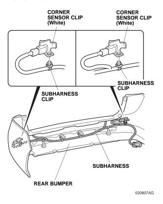
27. Secure two subharness clips to two holes on the rear bumper as shown.
