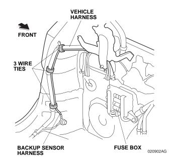
46. Route the backup sensor harness 2-pin connector along the vehicle harness.
