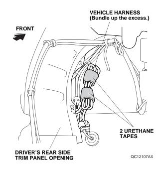
74. Secure the vehicle harness to the backup sensor harness and vehicle harness with two wire ties as shown.
