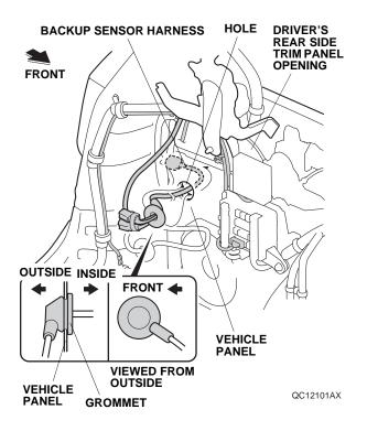
65. Route the backup sensor harness 8-pin connector, and secure the clip on the backup sensor harness 8-pin connector to the hole on the vehicle panel.
