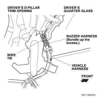
51. Route the backup sensor harness along the vehicle harness, and secure it to the vehicle harness with one wire tie as shown.
